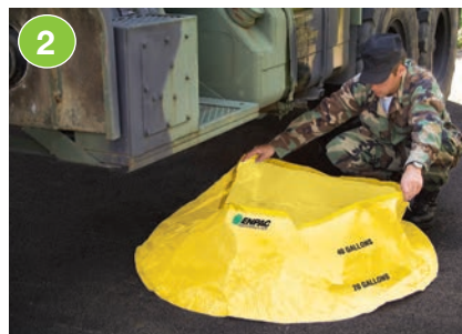
Step 2: Position pool underneath spill source.
