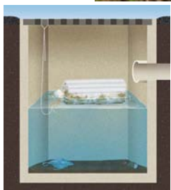
Skimmer floats while absorbing oils without taking in water.
