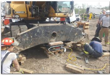
Use MatJacks under the most adverse conditions to re-locate, position or remove obstacles, even odd-shaped loads to make entry for Rescue possible. MatJacks air lifting bags are always ready to serve.
